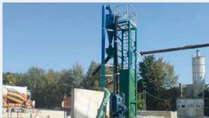
Cyclone deployed for fine sand recovery from the waste water of a gravel plant Feed approx. 200 m 3 /h, solids up to 15 t/h, separating cut at approx. 0.063 mm
