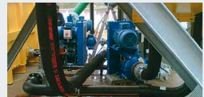
Pumps for STICHWEH sand classification – the pumps deliver water/solids mixtures from a screen underflow in the cyclones.
