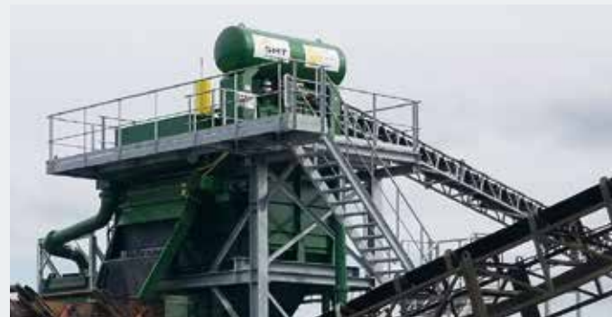
Jig Type 2500 SG, Location: Denmark Output 170 t/h, Grain size 2 – 32 mm Separation of constituents harmful to properties of concrete. The discharged light materials are drained through a dewatering mesh screen and conveyed to a tip.
