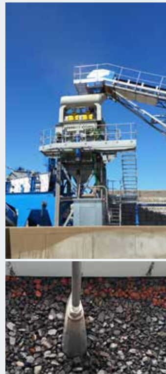
SSS Jig (Jig, approx. 1100 mm) Location: Hawaii/Oahu The particular challenge: separating red pumice from black crushed basalt. It was only when a jig was deployed that it became possible to achieve very good material yields: grain size approx. 6 – 38 mm at a throughput rate of 80 to 100 t/h.
