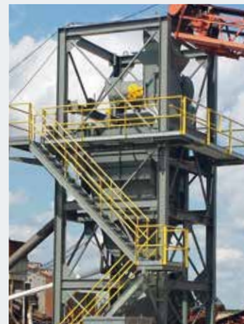
Jig Type 2500 SG, Location: Denmark Output 170 t/h, Grain size 2 – 32 mm Separation of constituents harmful to properties of concrete. The discharged light materials are drained through a dewatering mesh screen and conveyed to a tip.
