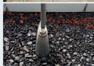
*A view of the material bed shows the process of separating the acceptable material (black crushed basalt) from the rejected material (red pumice).*
