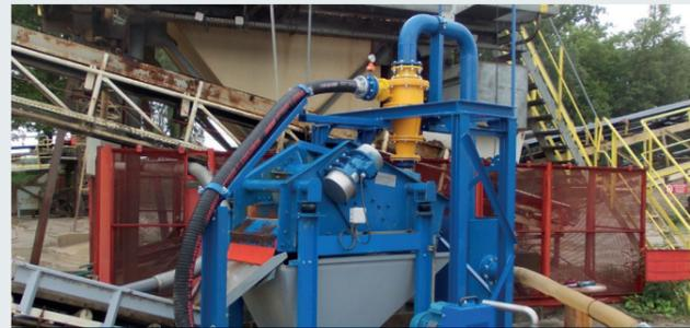
Cyclone deployed for **sand recovery from waste water** (from conveyor belt cleaning)
