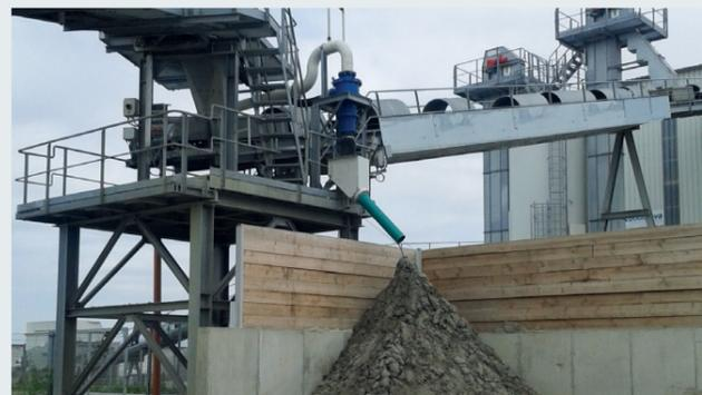
Cyclone deployed for **sand recovery from waste water** (from a log washer)
