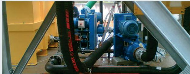
Underflow screening machine, cyclones and pumps deployed for **sand classification**, for every 100 m<sup>3</sup>/h
