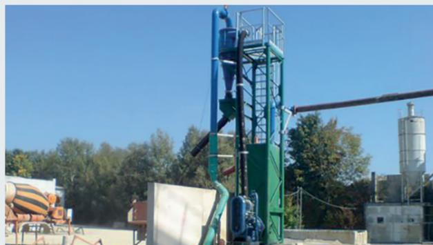
Cyclone deployed for **fine sand recovery from the waste water** of a gravel plant
